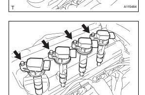
(b) Remove the 4 bolts and 4 ignition coils.
