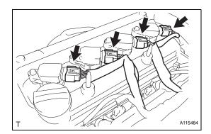
(b) Connect the 4 ignition coil connectors.
